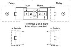
Note: Use Relays and Switches that have high contact reliability because the current flowing from terminals 1 or 3 is as small as approx. 10 µA.
