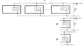
Note: H (Reset ON) level must be 4.5 V minimum.
