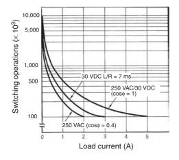
Reference: A maximum current of 0.15 A can be switched at 125 VDC ( $\cos \phi = 1$ ) and a maximum current of 0.1 A can be switched if L/R is 7 ms. In both cases, a life of 100,000 operations can be expected.
