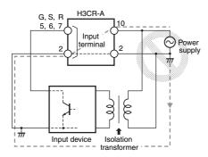
The H3CR-A $\Box$ /-A $\Box$ S/AP's power supply terminal 2 is a common terminal for input signals to the Timer. Do not disconnect the wires on terminal 2, otherwise the internal circuitry of the Timer will be damaged.
