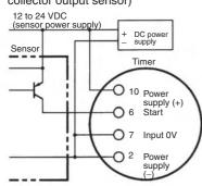
Operates with PNP transistor ON
