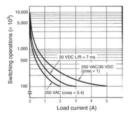
teference: A maximum current of 0.15 A can be switched at 125 VDC (cosφ = 1) and a maximum current of 0.1 A can be switched if L/R is 7 ms. In both cases, a life of 100,000 operations can be expected.
