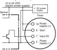
Operates with NPN transistor ON
