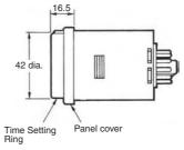
Dimensions with Front Connecting Socket P2CF-08-□/P2CF-11-□
