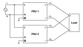
Fig. 4 Parallel Operation Connection Diagram
